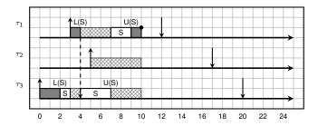
• Priority Inheritance consisting in giving the locking tasks the priority of the locked task
