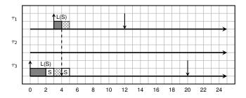
• Priority Inheritance consisting in giving the locking tasks the priority of the locked task
