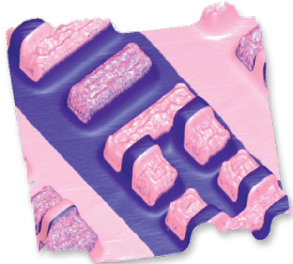
Accurate 2D dopant profiling on SRAM sample using Dark Lift SCM. Image size 15µm.
