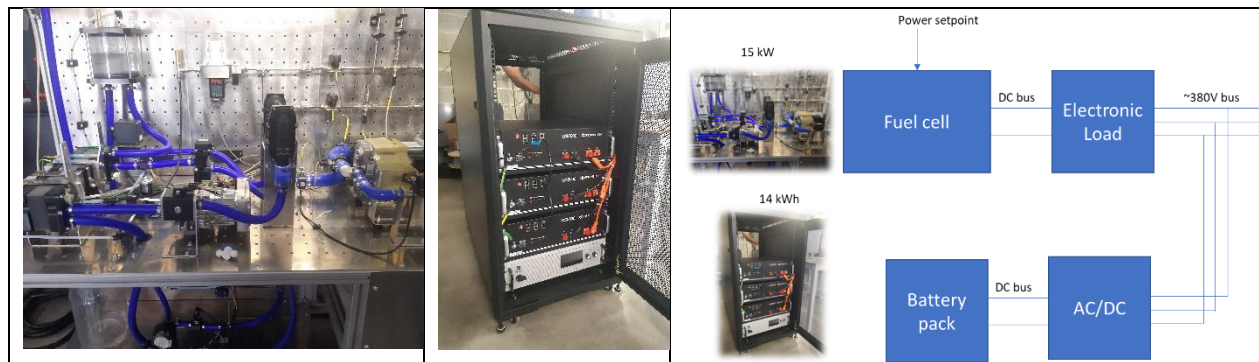
Figure 1: The Hybrid Fuel Cell test bench available at the LAMIH (Left : fuel cell system. Center: battery pack. Right: schematic)
