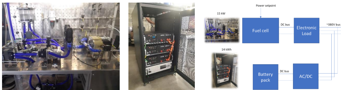
Figure: Hybrid fuel cell test bench at LAMIH-CNRS (Left : fuel cell system. Center: battery pack. Right: schematic).
